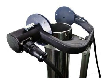
**Caution:** Ensure the sensor head has been powered on and self-calibrated before affixing the sensor head to the exhaust. If you self-calibrate the unit while the sensor head is in the flow of exhaust, the equipment will see the exhaust, think the exhaust is the normal dust in the air, and call it zero.
